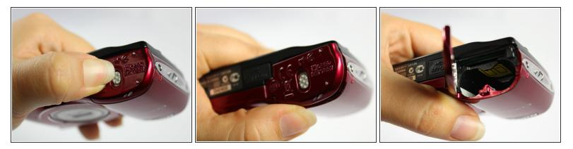
• Remove the batteries from the battery compartment by sliding the white battery compartment switch up and then move the panel toward the right.
