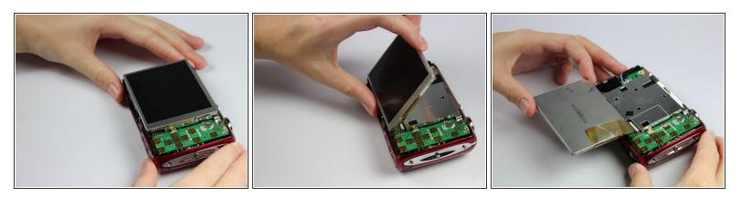
Carefully flip over the LCD screen onto its front. Pull the top of the LCD screen toward you keeping the bottom of it inside the camera.
