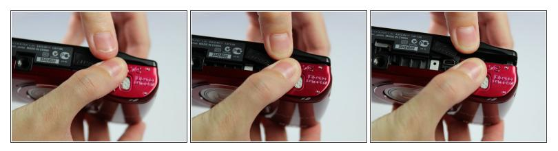
Using your hands, open the camera slightly by using the indentation above the camera compartment.
