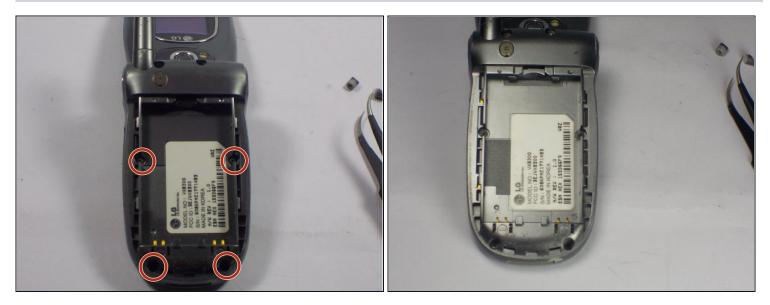
• Use a Phillips #00 screwdriver to remove all four 3mm screws from the back of the phone.
