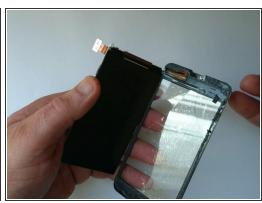
The display edges are glued to the glass with adhesive tape.
