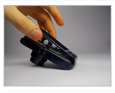
Remove the shell the from the back of the camera.
