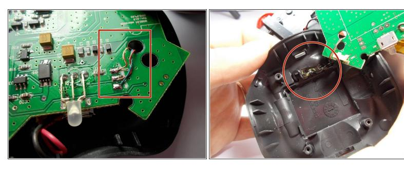
Locate the audio wire beneath the circuit board that is adjacent to the battery component on the very bottom layer of the device.
