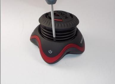
Remove the four 12 mm Phillips screws from the enclosure.
