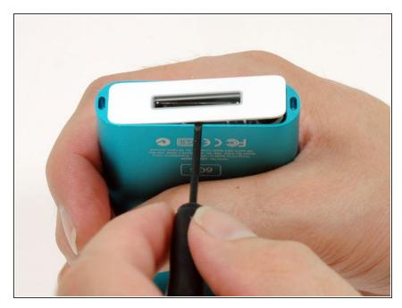
Carefully insert a small flathead screwdriver or <u>Jimmy</u> in the seam between the metal casing and white plastic bottom Use the screwdriver to pry up the white plastic bottom bezel. Be careful not to damage the soft plastic with your screwdriver.
