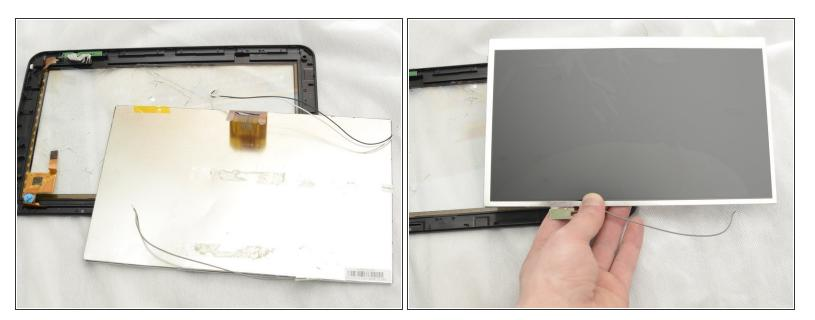
• The LCD can now be removed from the plastic tablet housing.
