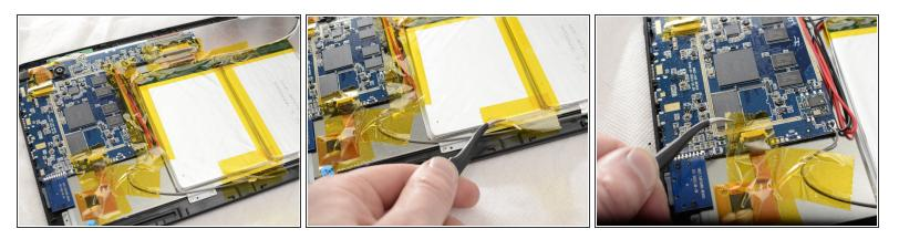
• Remove the non-conductive tape located on the battery and motherboard assembly.
