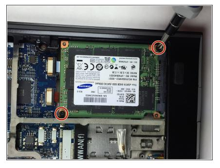
Unscrew the two 4.10x4.05 mm screws holding the SSD in place.
