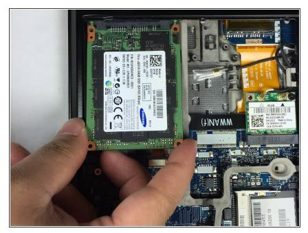
Using your finger and thumb lift the hard drive out of the computer but do not disconnect the attached connector to the computer.
