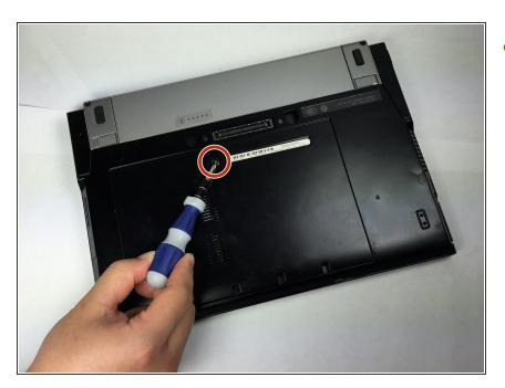
Use PH0 screwdriver to unscrew the 4.49x7.88 mm screw in the middle of the back panel.
