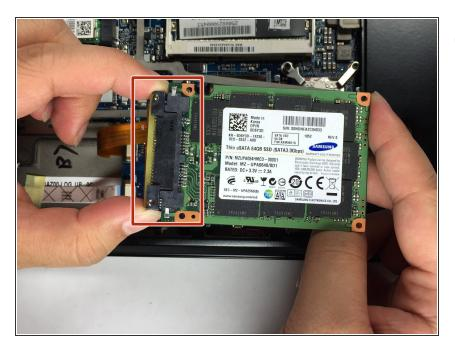
By applying pressure to the sides of the connector, pull the connector apart from the SSD.
