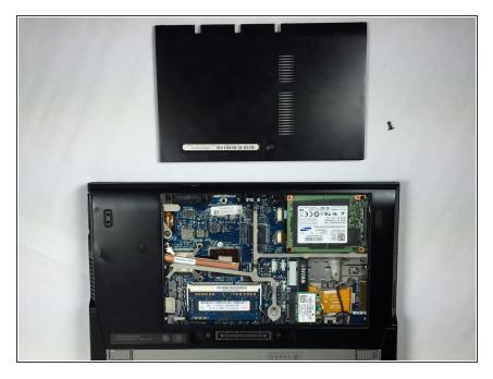
Remove panel and screw from the device. This opens up the main board of the device.
