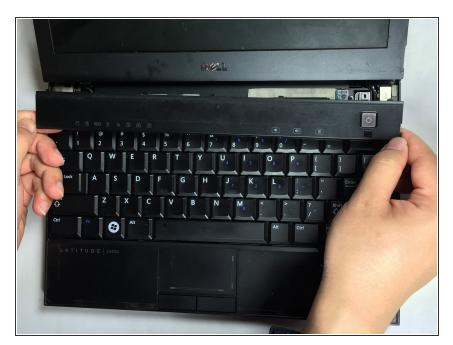
Once out of place, position your thumbs under the bottom of the panel and pull upwards.
