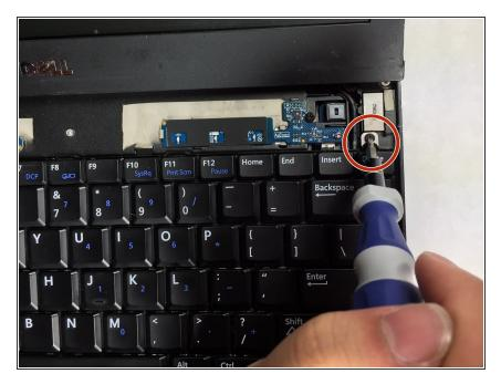
Use a PH00 screwdriver to unscrew the screw.
