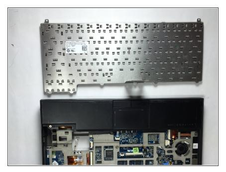
Completely lift the keyboard from the device, as they are now disassembled.
