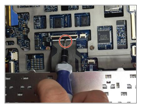
Use a flat head screwdriver to flip the keyboard connector up. This will allow you to disconnect the keyboard and remove it.
