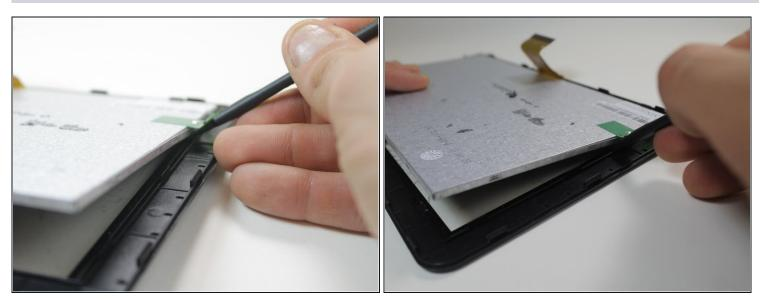
• After removing the motherboard, use the black nylon spudger to pop the screen out of the housing holding it to the front of the screen case.
