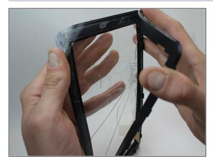
• Pull the thin plastic screen casing apart and you can remove the damaged screen.
