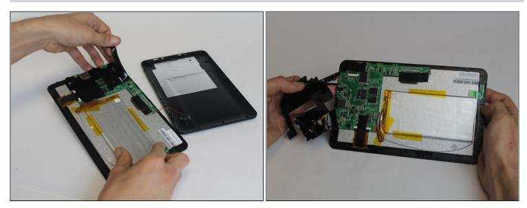
• Begin removing the black tape covering the motherboard inside the tablet.
