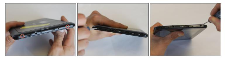
• To begin, locate the two 4.9mm Phillips #00 screws at the top corners of the case and remove them.
