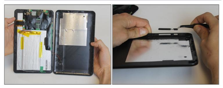
• Carefully place the bottom lid next to the screen case. The power/speaker buttons should be visible at the corner of the lid. Remove the buttons with the <u>tweezers</u>.
