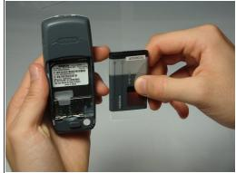
Using your fingernail, pry the back of the battery upwards and pull out.
