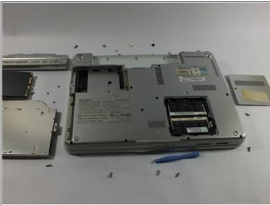
Using a #00 Phillips screwdriver, remove the screws
