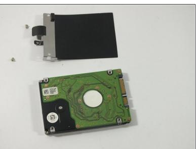
Using a #00 Phillips screwdriver, remove the screw
