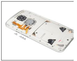
• Remove securing bracket and side buttons.
