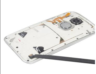
• Release power connecting flex connector and battery connector.
