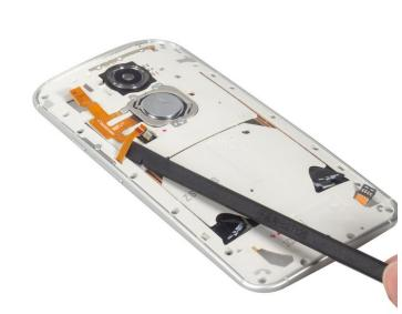
• Release power flex connector from connecting flex.
