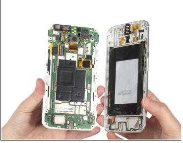
Twist off all 18 black torx screws and remove the middle housing from front assembly.
