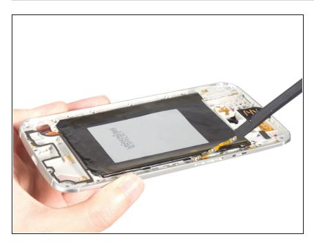
• Pry up and remove the power flex.
