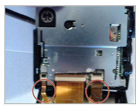
Once the back has come off, detach the data strips from the back part of the camera, or from the main part of the camera if the replacement part does have the data strips.
