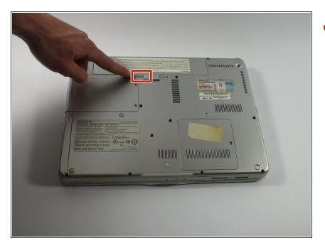
Put the lock switch to the left to unlock the safety lock.
