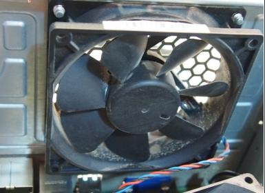
Remove the four screws on the outside of the case that hold the fan in place.
