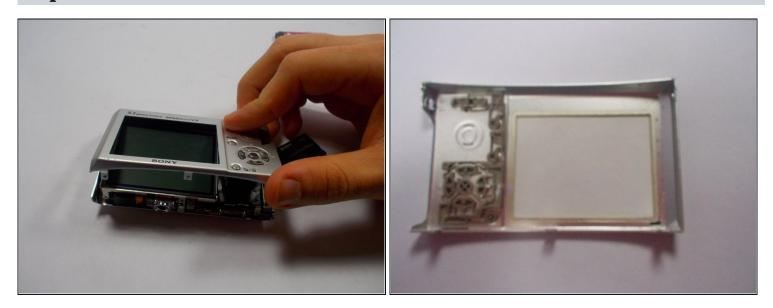
• Remove the front case by carefully pulling it off from the camera.
