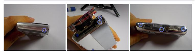
Use a Phillips #000 to remove all 6 exterior screws from the casing.
