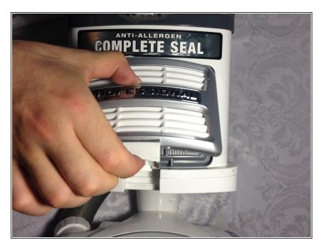
Press up on the latch and remove the front vent
