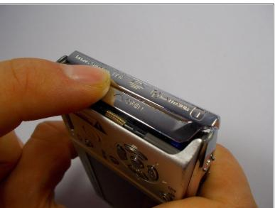
Push open the sliding cover to access screws.
