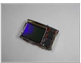
Remove the back cover panel from the rest of the camera.
