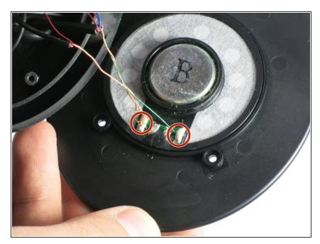
Desolder the colored wire and copper wires.
