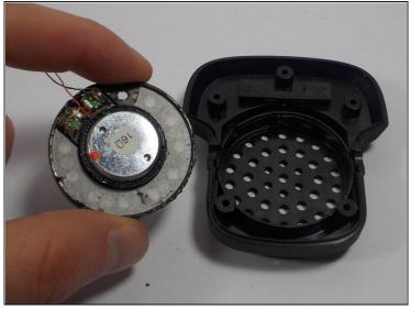
• Remove the speaker from its circular shaped slot.
