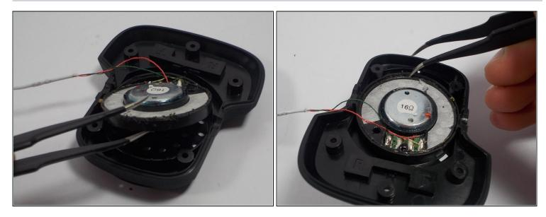
• Insert your new speaker into the circular shaped slot located on the speaker cover.
