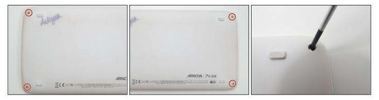
• Remove four 5 mm Phillips #00 screws from each corner of the tablet.
