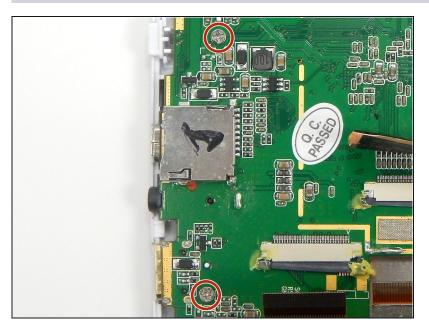
Remove the two Phillips #00 screws from the motherboard.
