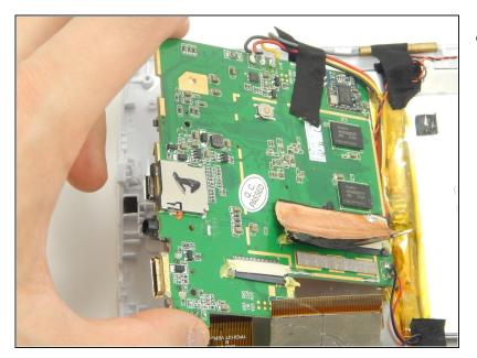
• Gently lift up the motherboard and reorient it in a more efficient manner in order to locate the desired components.
