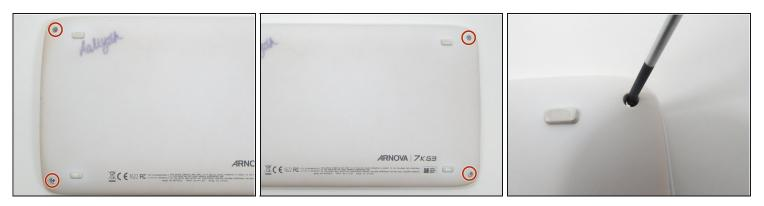
• Remove four 5 mm Phillips #00 screws from each corner of the tablet.
