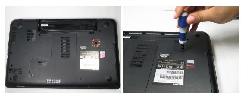
• Remove the 3mm Phillips #00 screw holding the keyboard in place.
