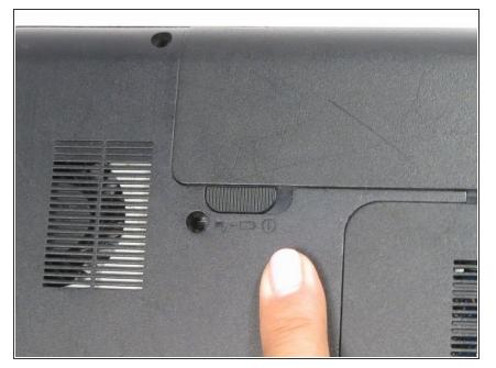
• Release the locking mechanism by switching the left slider to the left.
