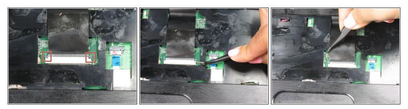
• Using tweezers, push up the two black switches on either side of the ZIF connector.
