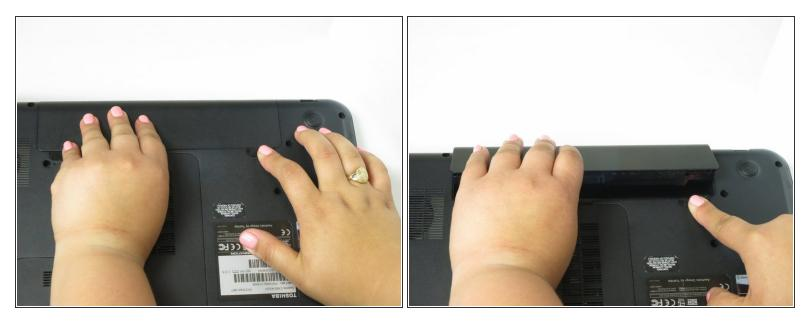
• Slide the right slider to the right, and simultaneously, pull the battery out at a diagonal angle.
