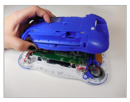
Carefully separate the back panel from the front panel revealing the motherboard connected to the front panel.
