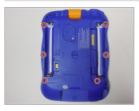
Remove the six 7.6mm screws found in the battery compartment using a PH00 screwdriver.
