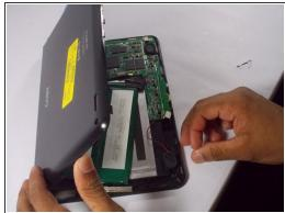
Potential for device damage. Be careful not to break the inner plastic tabs while pulling the back cover off.
