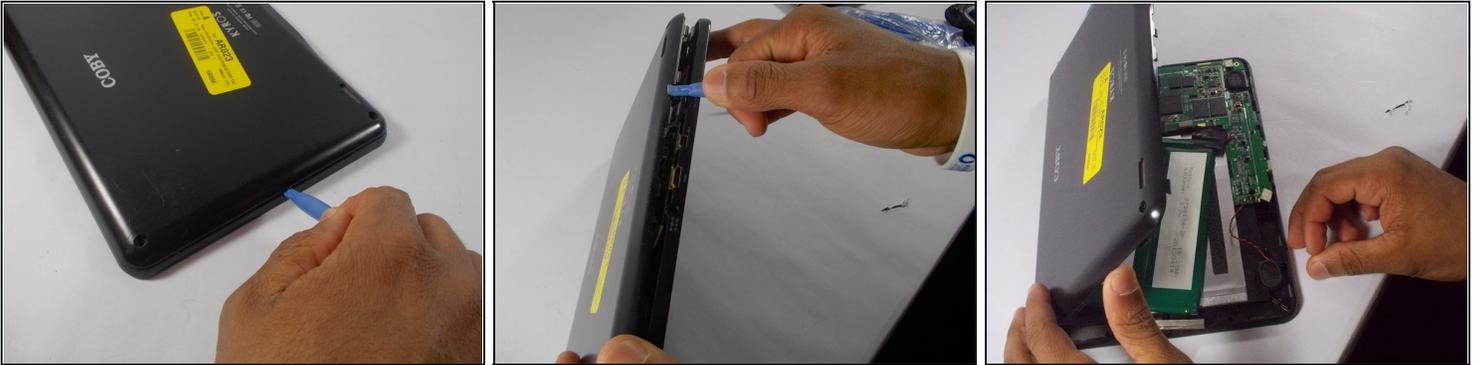
**⚠** When removing the back cover, be careful not to break the inner plastic tabs.
