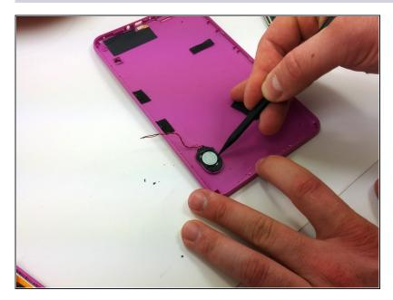
• Pry the speaker gently out of its plastic enclosure using a spudger.
