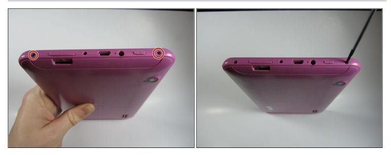
• Use a Phillips #00 screwdriver to remove both 4.1 mm screws at the top of the device which hold it together.
