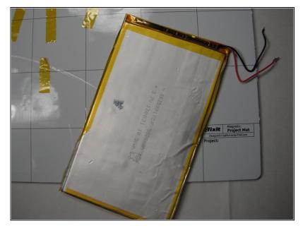
The battery should now be separated from both the screen and circuit board
