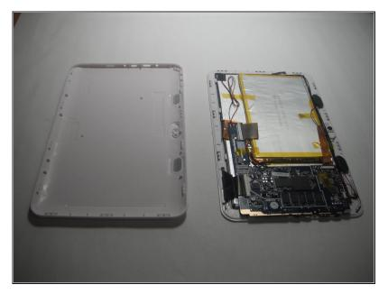
Remove the back cover with your hands once all points have been unlatched. It should separate completely from the screen that contains the battery and chip components.
