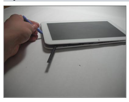
Place the spudger in an open space to keep the back case from shutting while you continue to slide the opening tool.
