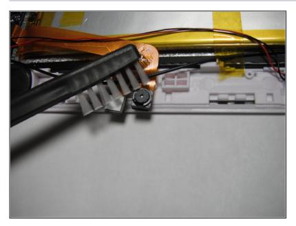
Brush the surfaces of the cameras to remove any debris that is present.
