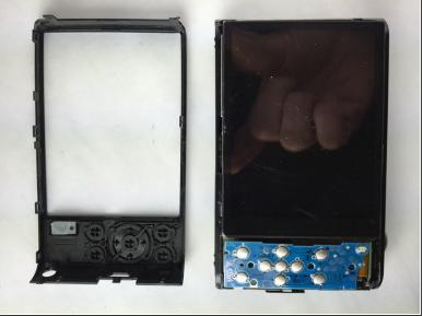
Remove the back case of the camera carefully.
