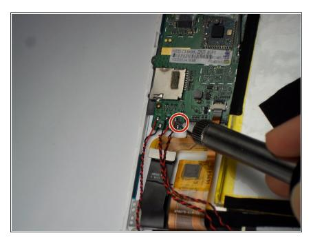
You will need a soldering/desoldering kit to <u>desolder</u> the 2 leads where the microphone connects to the circuit board.
