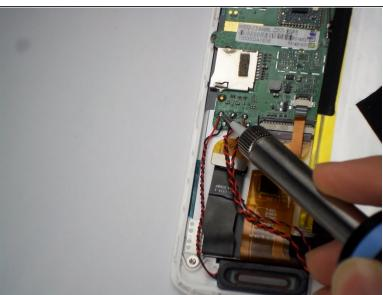
You will need a soldering/desoldering kit to <u>desolder</u> the 4 leads where the speakers connect to the circuit board.
