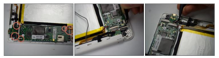
• After removing the top panel, battery, speakers, microphone, and front camera from the tablet, you will also need to use the <u>tweezers</u> to remove the connectors indicated in the same method as the previous step.
