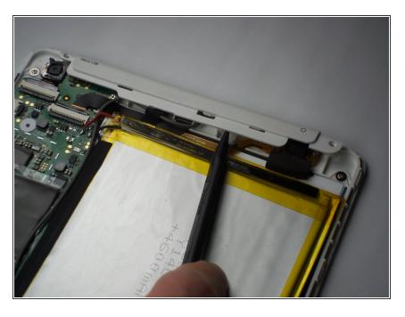
Once unscrewed, use a spudger to pop the panel off by wedging it underneath the panel.
