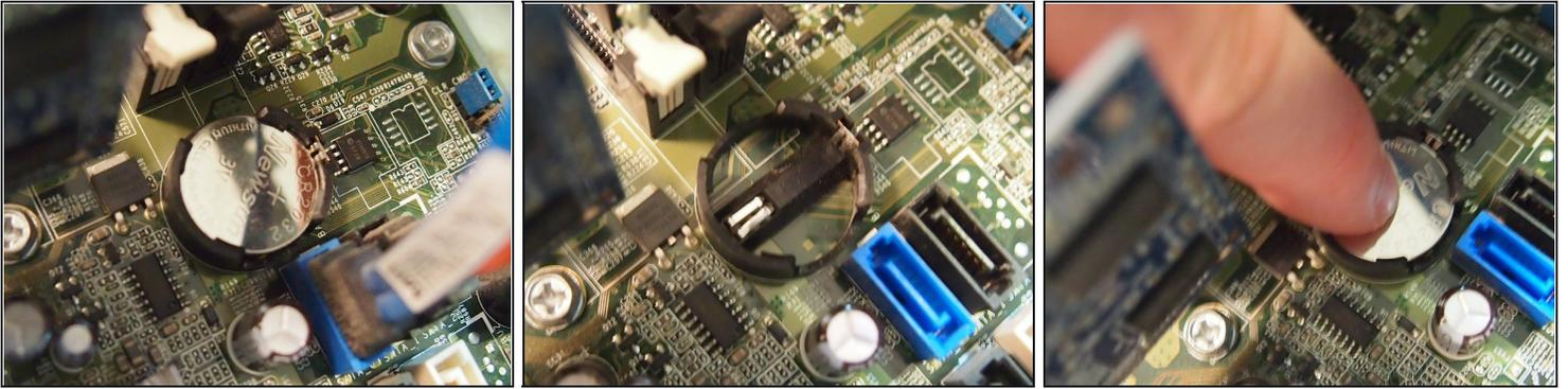
**⚠ The CMOS battery has to be removed properly to avoid damaging the motherboard.**
