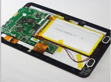
Lift the back cover from the body of the device to expose the internal components.
