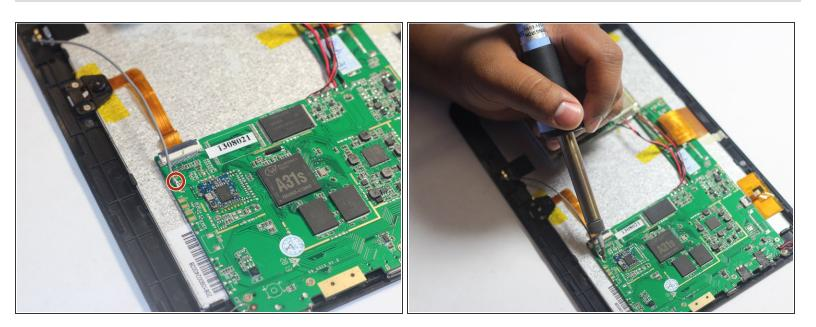
Desolder the FM antenna from the motherboard.
