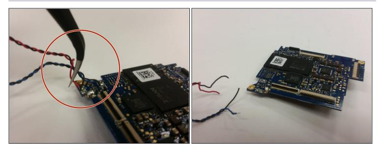
• Desolder the four wires from the old motherboard.
