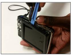
• Use the Plastic Opening Tool and your finger to pry off and remove the external cover.
