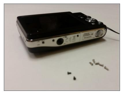
Remove the six 3 mm external screws from the camera base using the Phillips #000 screwdriver.
