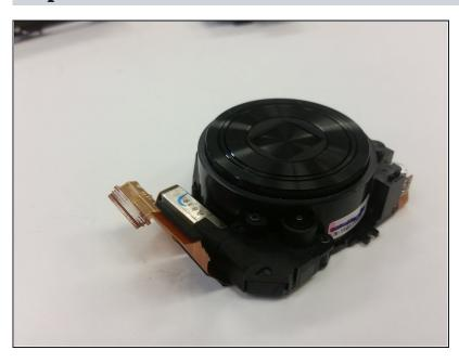
You have now separated the lens unit. Replace it with a functional lens unit at this stage, and reassemble the device.
