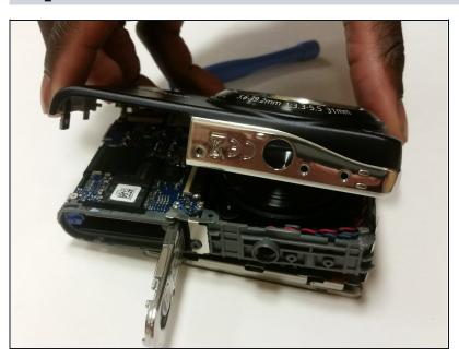
Remove the front cover of the camera using your fingers and a plastic opening tool.
