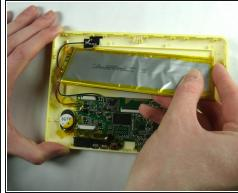
Gently remove tape from the side of the battery connecting to wires and circuits.
