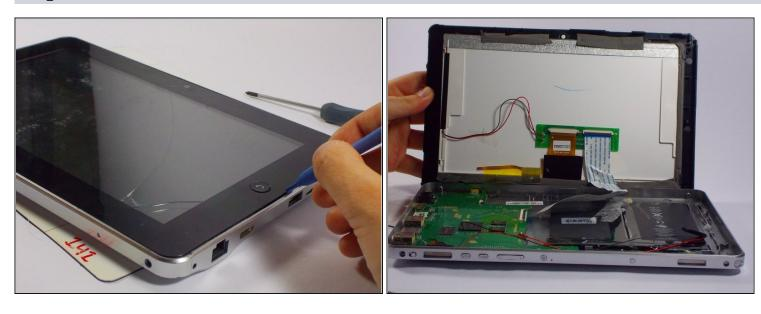
• Use the opening tool to pry the screen from the case applying pressure at each of the four corners of the screen.
