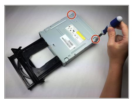
Using the Phillips Head #2 screwdriver, unscrew the two 8.5 mm screws located on the bottom back of the chassis.
