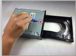
Use a plastic opening tool to push the three tabs located on the right, left, and bottom side of the outer chassis to loosen the faceplate off.
