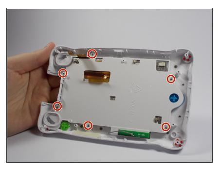
Remove the 6 screws that hold the screen in place
