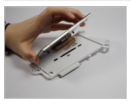
Separate the screen from the plastic casing.
