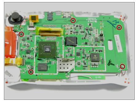
Use the Philips #00 screwdriver to remove the 5 screws from the motherboard
