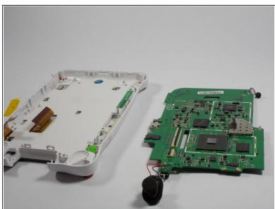
Lift motherboard to separate it the from the case shell.
