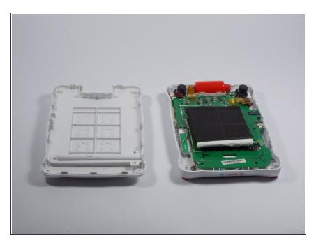
After loosening the back cover, remove it from the device so you can get at the innards.
