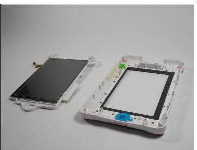
Remove the screen from the front casing
