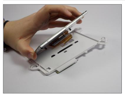
• Separate the screen from the plastic casing.
