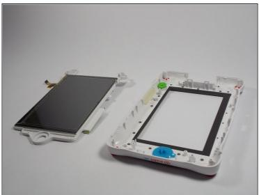
Remove the screen from the front casing
