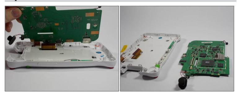
• Lift motherboard to separate it the from the case shell.
