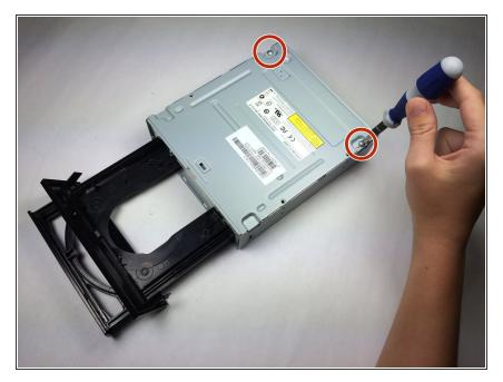
Using the Phillips Head #2 screwdriver, unscrew the two 8.5 mm screws located on the bottom back of the chassis.
