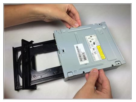
• Remove the bottom plate by lifting it off the device.
