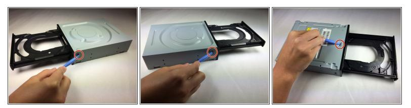
• Use a plastic opening tool to push the three tabs located on the right, left, and bottom side of the outer chassis to loosen the faceplate off.
