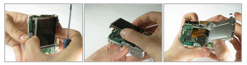
• Carefully lift the LCD screen away
