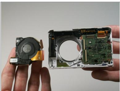
Remove the lens assembly from the camera.
