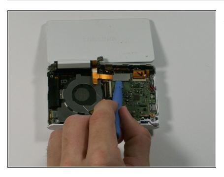
Use plastic opening tool to disconnect screen connector from the control board.
