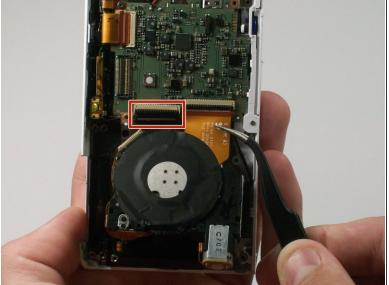
• Use a pair of tweezers to flip up the black retaining bar on each of the two ZIF connectors.
